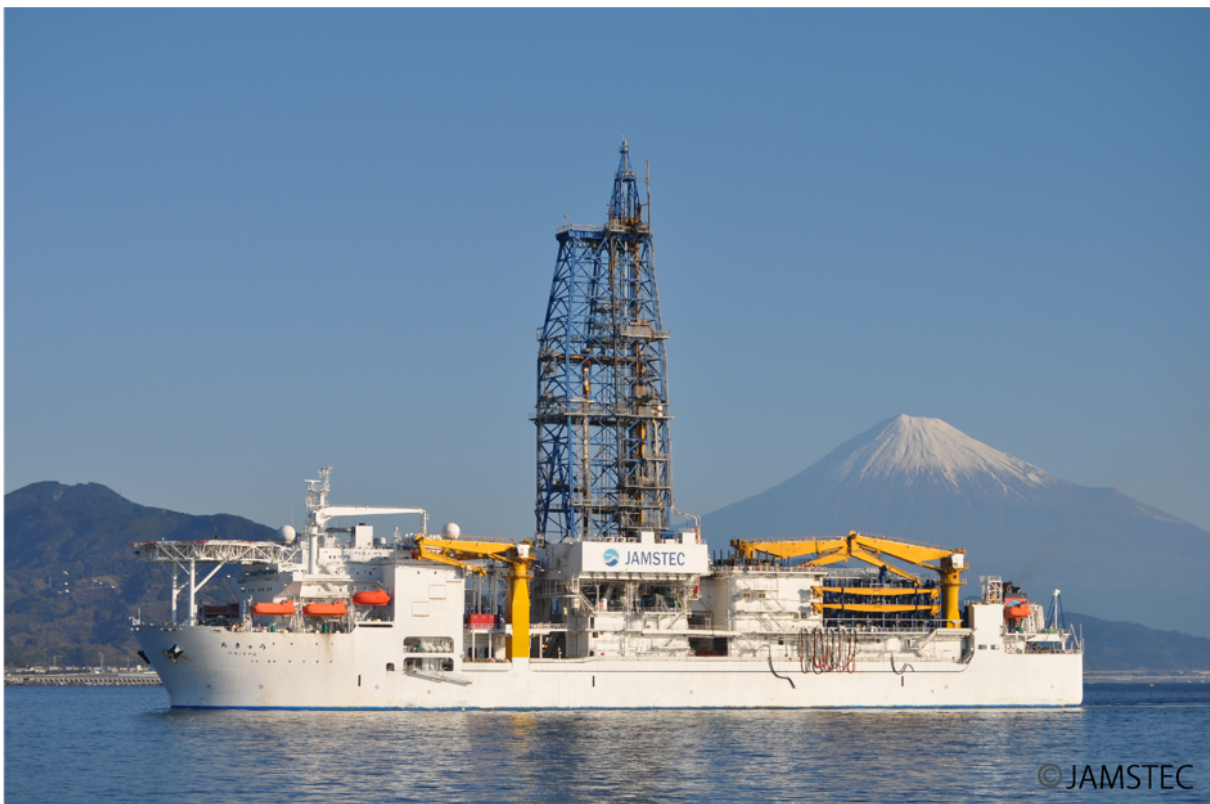
Drilling vessel CHIKYU. Length: 210 m, Height: 130 m, Gross tonnage: 56,752 tons
